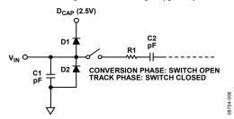
Figure 22. Equivalent Analog Input Circuit
