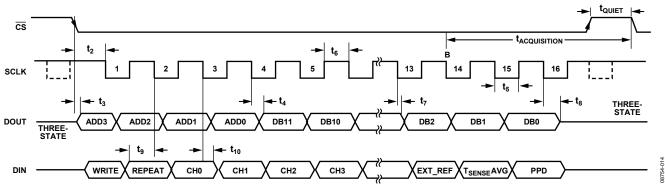
Figure 30. Serial Interface Timing Diagram
