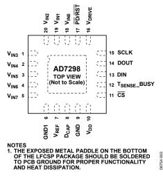
Figure 2. Pin Configuration
