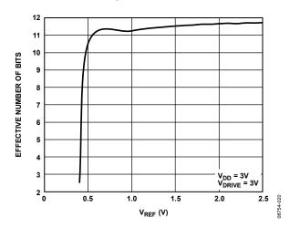
Figure 8. Effective Number of Bits vs. V<sub>REF</sub>
