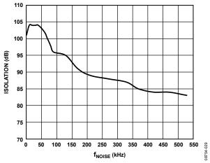
Figure 12. Channel-to-Channel Isolation,  $f_{IN} = 50 \text{ kHz}$
