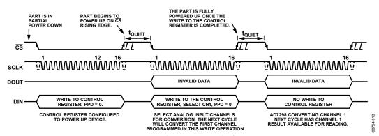
Figure 29. Partial Power-Down Mode of Operation
