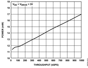
Figure 18. Power vs. Throughput in Normal Mode with  $V_{\text{DD}} = 3 \text{ V}$
