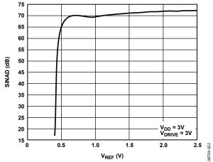
Figure 14. SINAD vs. Reference Voltage
