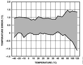
Figure 15. Temperature Accuracy at 3 V
