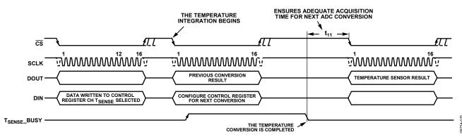
Figure 31. Serial Interface Timing Diagram for the Temperature Sensor Conversion
