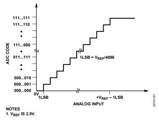
Figure 23. Straight Binary Transfer Characteristic
